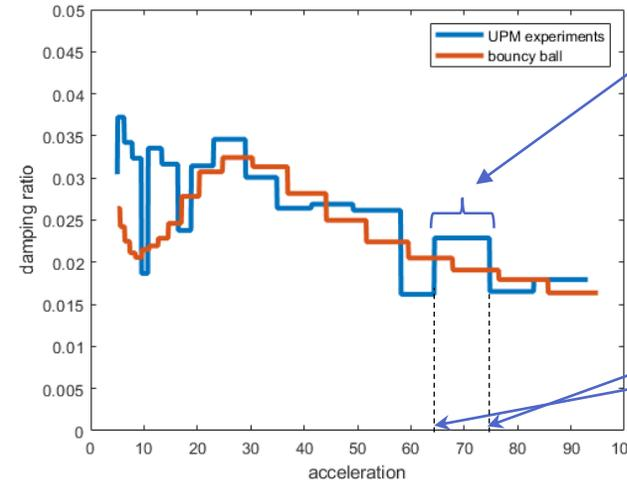
Damping ratio assumed **constant** between two consecutive peaks of the acceleration amplitude
