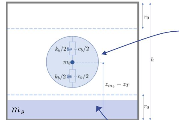
**Vertically bouncing ball** able to emulate the vertical sloshing impacts mechanism and dissipation
