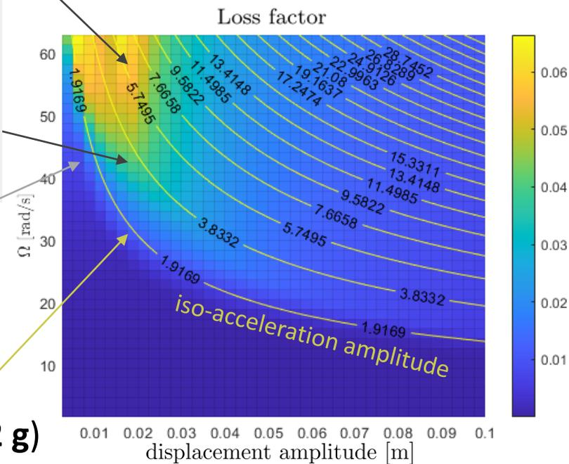
The lack of impacts before the border leads to **no energy dissipation**
