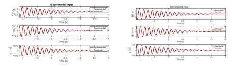
Acceleration, velocity and position results match the experimental measurements.
